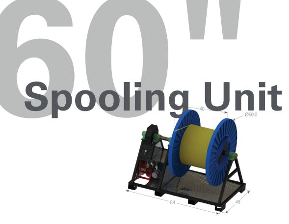
DataCan offers either an Air Spooler or Hydraulic Spooler, both of which are used to run conductor cable into the well. Both spoolers come with through spool communication via two conductor split ring. The spooling units have up to 60" diameter spool capacity and a split bearings and shaft for easy spool changes.
